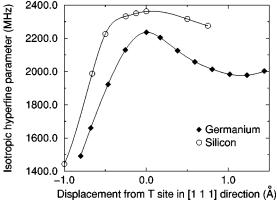
FIG. 9. The variation in the isotropic hyperfine parameter along the [1 1 1] direction at the T site in silicon (54-atom supercell) and germanium (16-atom supercell). A positive displacement indicates movement towards the hexagonal site. The lines are guides to the eye.
