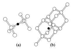
FIG. 1. The muon/proton at the bond-centered (a) and tetrahedral (b) sites in silicon. The dashed circles in (a) show the unrelaxed positions of the silicon atoms. These are not shown in (b) because the relaxations around the T site are negligible.
