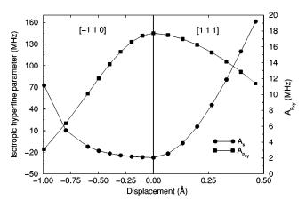
FIG. 8. Variation of the isotropic hyperfine parameter and the xy component of  $\mathbf{A}_p$  with displacement of the muon/proton from the BC site. The calculations were performed in silicon with the 16-atom supercell and the standard basis set. The lines are guides to the eye.
