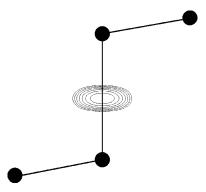
FIG. 4. The calculated potential experienced by the muon/ proton in the  $\{110\}$  planes for the BC site in silicon. The figure shows both of the NN and two of the NNN silicon atoms of the muon/proton with the bond lengths drawn to scale. The contours range from 0.1 to 0.7 eV in increments of 0.1 eV.
