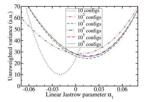
All-electron neon atom:  $\sigma_{u\alpha}^2$  plotted against a linear Jastrow parameter. Configurations are distributed according to square of Hartree–Fock wave function.
