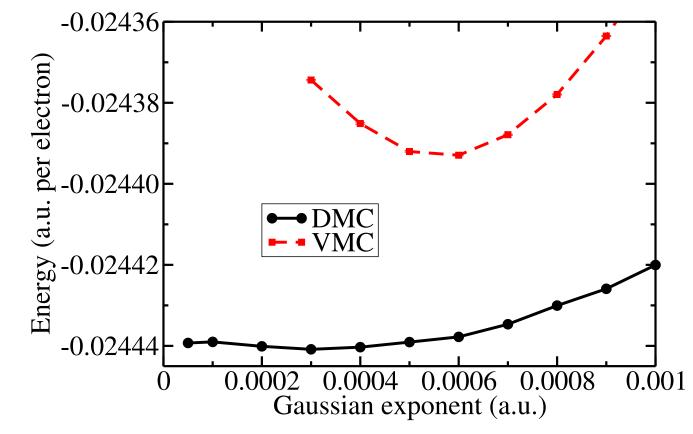
VMC and DMC energy of a 2D hexagonal Wigner crystal at  $r_s = 40$  a.u. against the Gaussian exponent in the orbitals.
