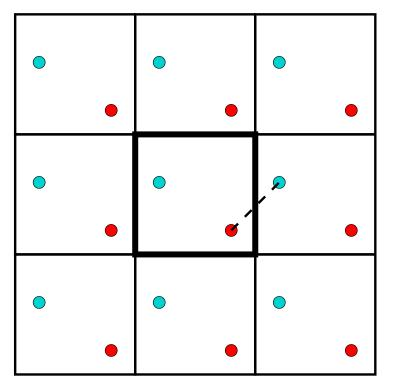
Minimum-image distance between **red** and **blue** particles in simulation cell. Used in evaluation of Jastrow factor.
